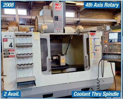
HAAS VF-4B CNC VERTICAL MACHINING CENTER
